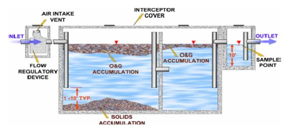
**REMINDER**: DEGREASERS, DETERGENTS, AND WATER EXCEEDING 140 DEGREES SHOULD <u>NOT</u> BE PASSED THROUGH THE GREASE REMOVAL DEVICES.
