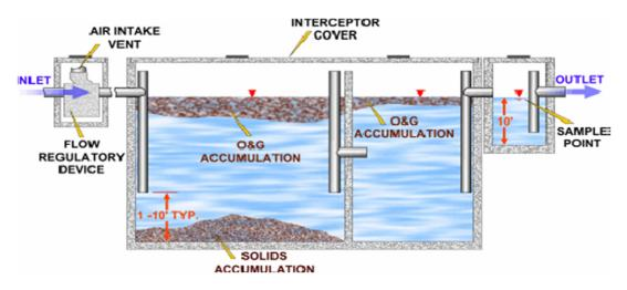
**REMINDER**: DEGREASERS, DETERGENTS, AND WATER EXCEEDING 140 DEGREES SHOULD <u>NOT</u> BE PASSED THROUGH THE GREASE REMOVAL DEVICES.
