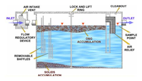
**REMINDER**: DEGREASERS, DETERGENTS, AND WATER EXCEEDING 140 DEGREES SHOULD <u>NOT</u> BE PASSED THROUGH THE GREASE REMOVAL DEVICES.
