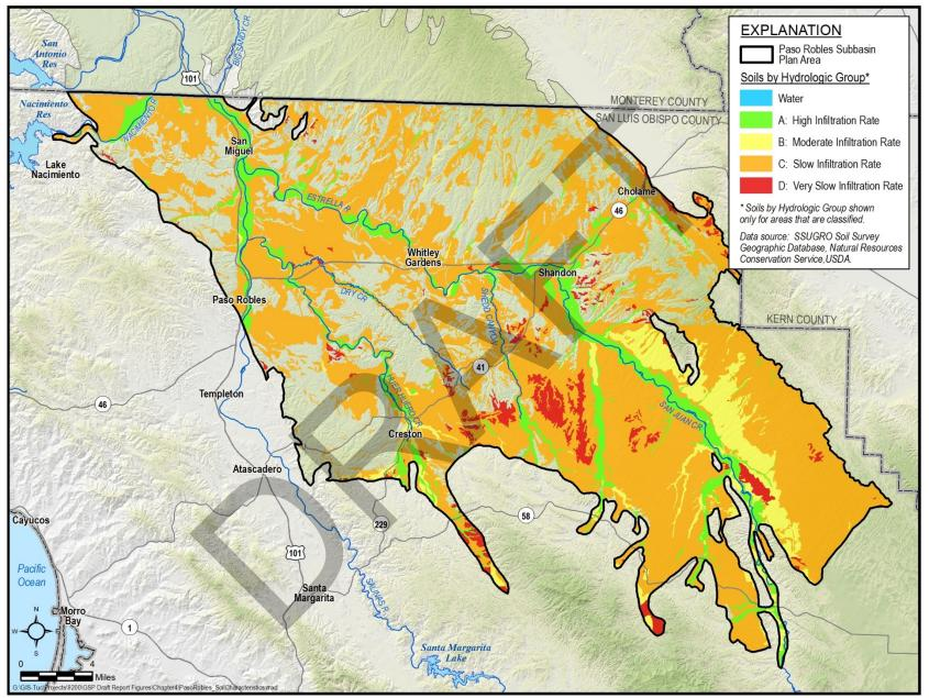
Figure 4-3. Paso Robles Subbasin Soil Characteristics
