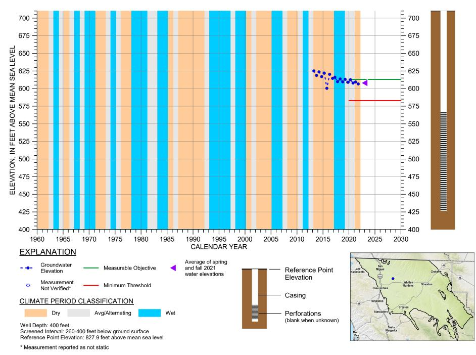
HYDROGRAPH OF MEASURED GROUNDWATER ELEVATION FOR 26S/13E-08M01
