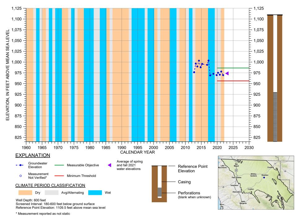
HYDROGRAPH OF MEASURED GROUNDWATER ELEVATION FOR 26S/15E-29R01
