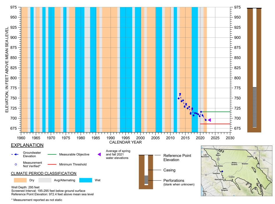
HYDROGRAPH OF MEASURED GROUNDWATER ELEVATION FOR 27S/12E-13N01
