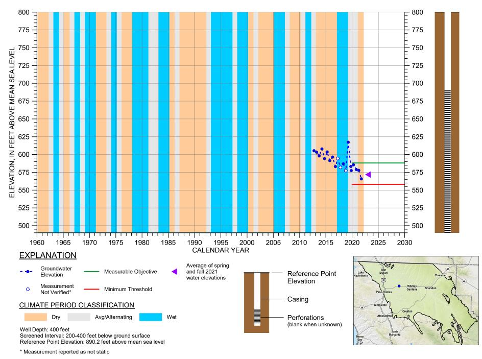
HYDROGRAPH OF MEASURED GROUNDWATER ELEVATION FOR 26S/13E-16N01
