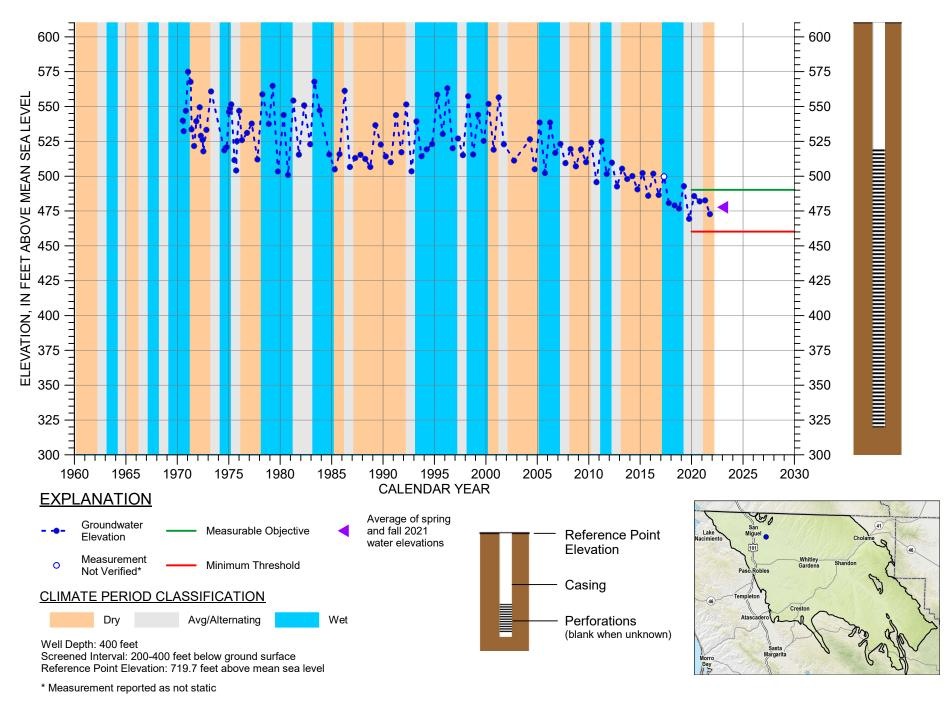
HYDROGRAPH OF MEASURED GROUNDWATER ELEVATION FOR 25S/12E-26L01
