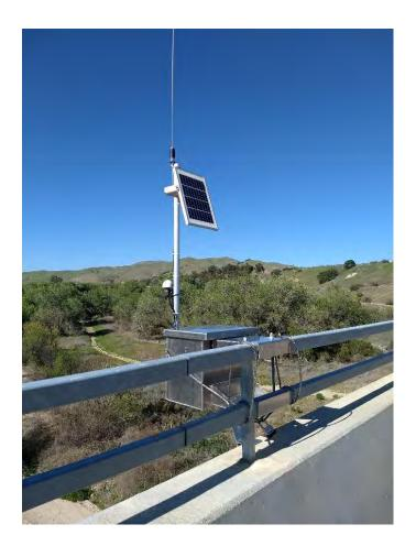
Figure 3. San Miguel (Salinas River) radar sensor stream gage installation
